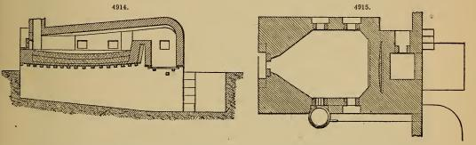
has a smaller number of working openings. The bottom is carried on bars of iron, and there is a small pit at the side arranged for the overflow of the regulus from the lead-pot. The furnace is usually lined with fire-brick cased with granite, and has the working bottom lined with slag. The hearth is very much sloped towards the small pits a.
